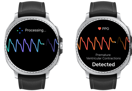
Figure 3 | Model efficiency and on-device inference: Sample on-device detections on Samsung Watch 8 device. Size, compute cost, memory footprint, and CPU latency (ms per sample, batch size 2048) measured over a 10s sequence at 100Hz.
